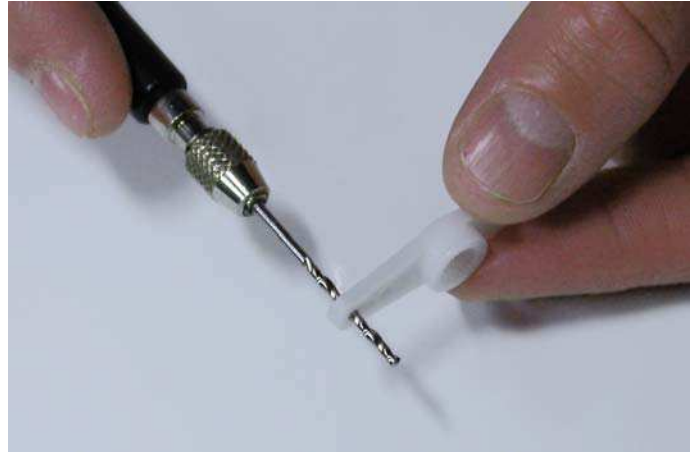
Fig.88: Widen the servo horn hole.
