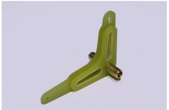
Fig.11: Glue the bellcrank to the reinforcements.
