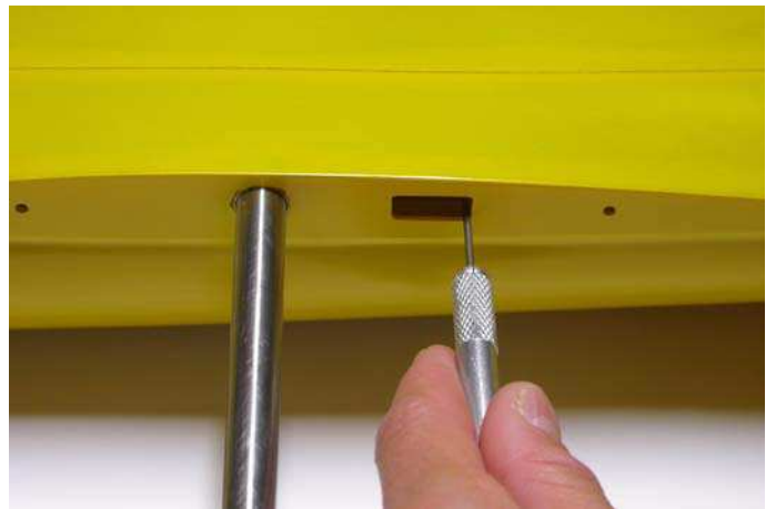
Fig.59: Trace the contour of the hole.
