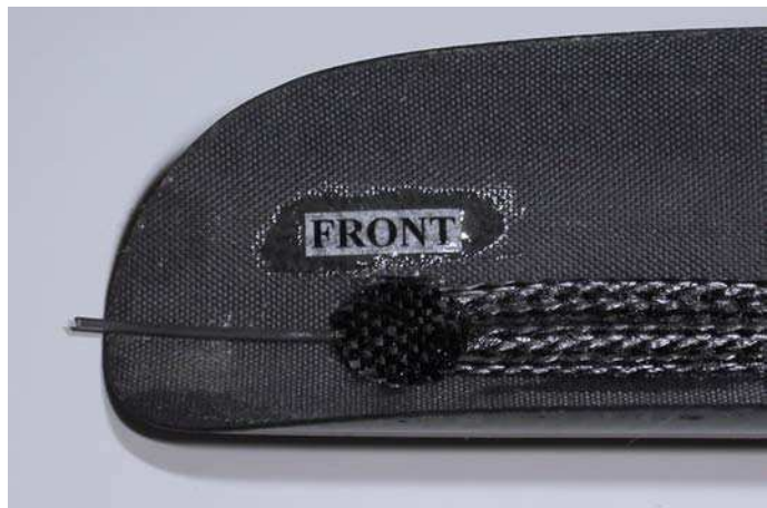
Fig.111: How to identify the canopy front side.
