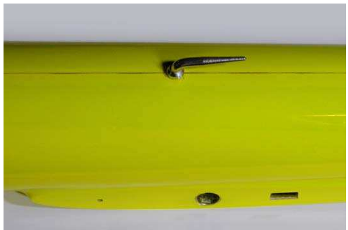
Fig.81: Screw the hook (oriented towards the tail).
