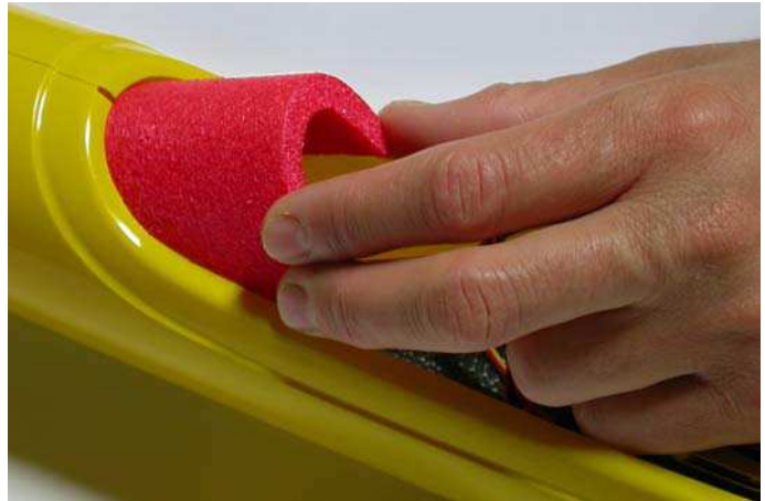
Fig.50: Insert the strip into the fuselage's nose.
