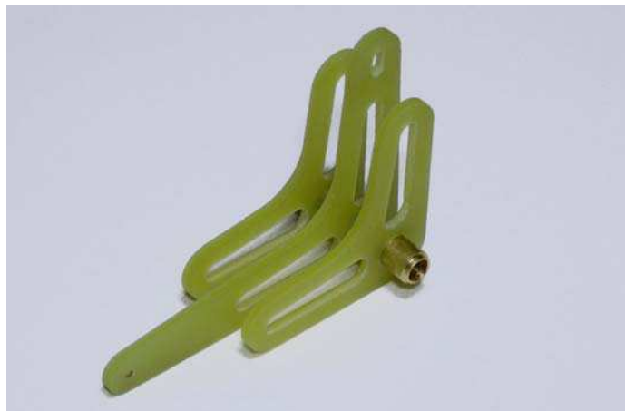
Fig.10: Insert the bush into the pieces.
