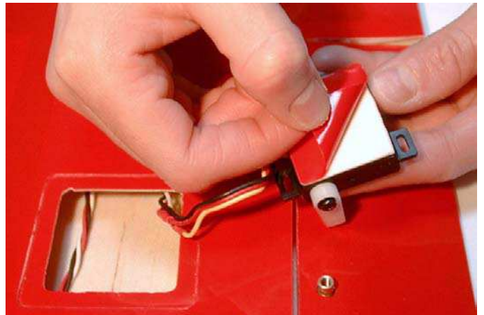
Fig.123: Apply the double adhesive plate.
