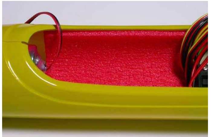
Fig.106: Insert the strip in fuselage.
