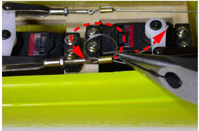
Fig.98: Make a ring with the end of the cable.
