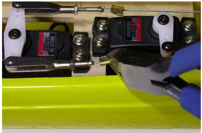
Fig.99: Squeeze the tube in more points.
