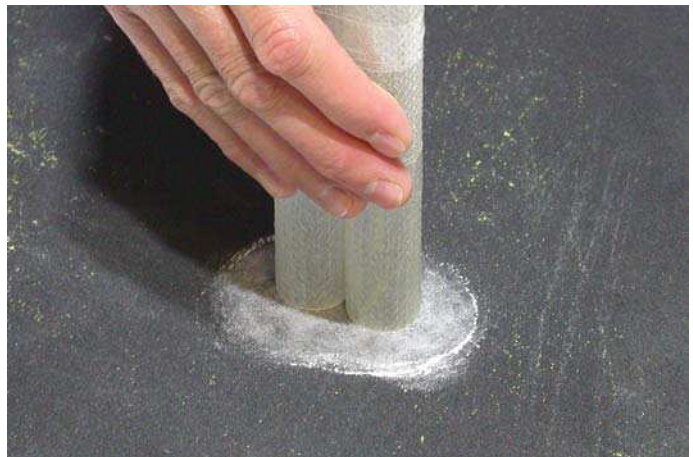
Fig.75: Level the two ballast hold tubes.
