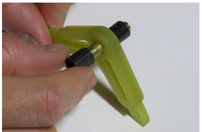
Fig.13: Mount the two spacers on the bush.
