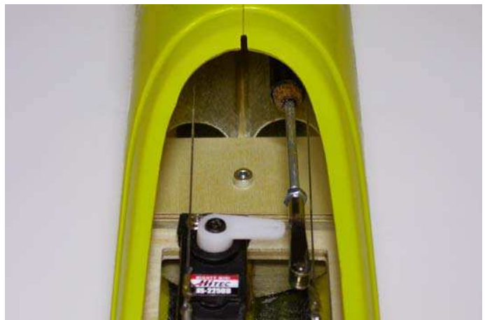
Fig.105: Ballast locking plate in position.
