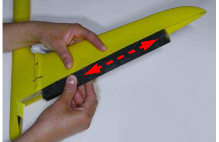
Fig.35: Remove the internal excess of glue.
