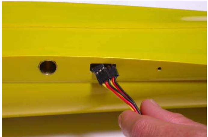
Fig.61: Inserting RX connectors.
