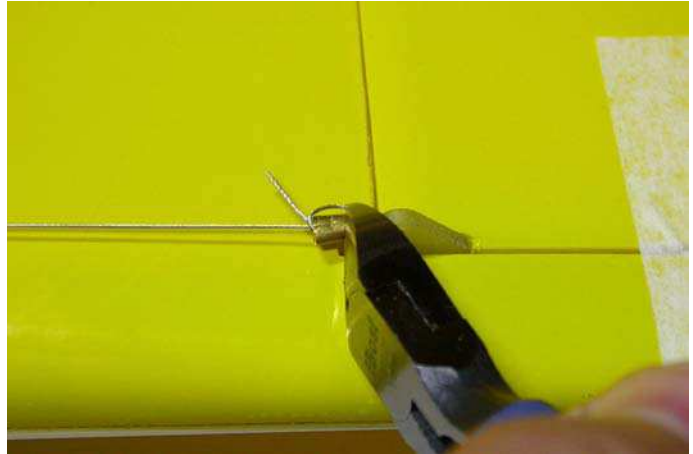
Fig.103: Squeeze the tube in more points.
