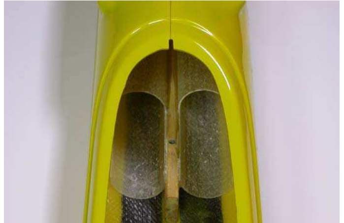
Fig.82: Ballast holding structure in position.
