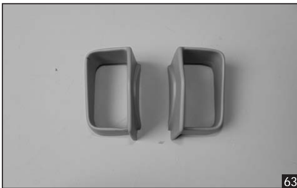
6. Glue the plastic inlet lip using C.A glue.
