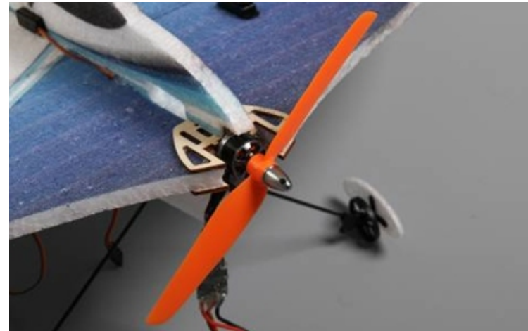
25. Fix the propeller on the motor through bullet nut.
