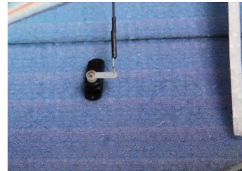
21. Install the Z bend on the servo arm after pushrod assembly.
