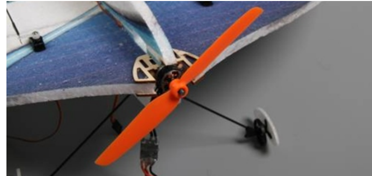
24. Install the propeller on the motor shaft.
