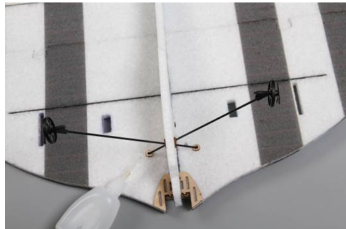
7. Cross the landing gear carbon pushrod to lower fuselage, put on the bottom surface of front wing, and fix with glue.
