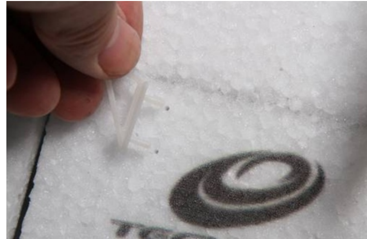
17. Install the plastic servo horn into the corresponding hole site of control surface
