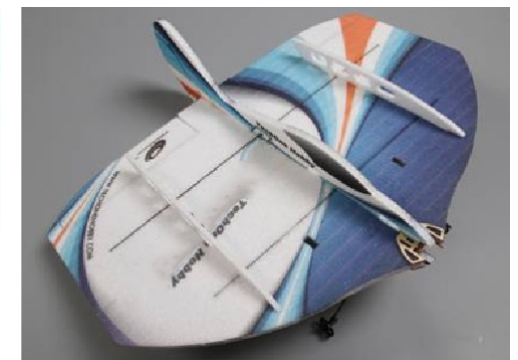
9. Put upper fences on the corresponding of the wing, then fix with glue, and make sure they are perpendicular to each other.
