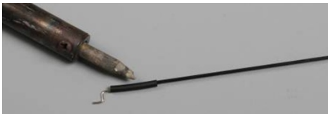
19. Fixed the Z steel through the shrink tube on the one head of the carbon pushrod of control horn, make sure to strengthen again with glue.
