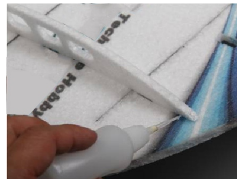
9. Put upper fences on the corresponding of the wing, then fix with glue, and make sure they are perpendicular to each other.
