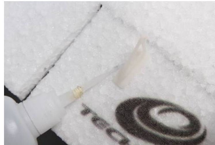
18. Place the servo horn well, then fix with glue
