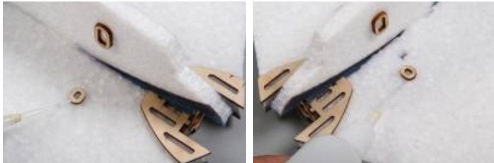
6. Fix the reinforced wood of landing gear on the corresponding slot of Front wing and lower fuselage with glue.
