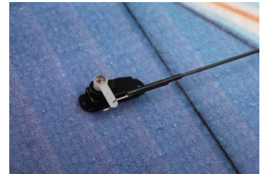
21. Install the Z bend on the servo arm after pushrod assembly.
