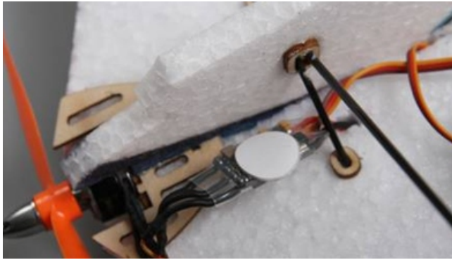
26. Tear one surface of round velcro and glue on the ESC.
