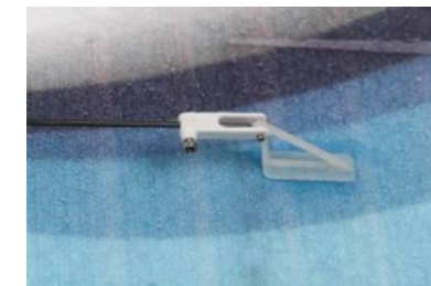
22. Install one head with clevis of assembled pushrod on the servo horn.
