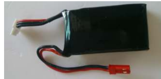
Battery: 350mah 7.4V lipo 20c
