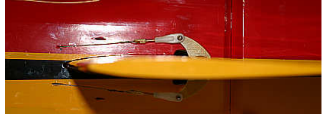
Picture 24: Elevator linkage / Icon Image
