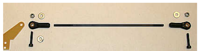
Picture 25: Elevator / Pushrod
