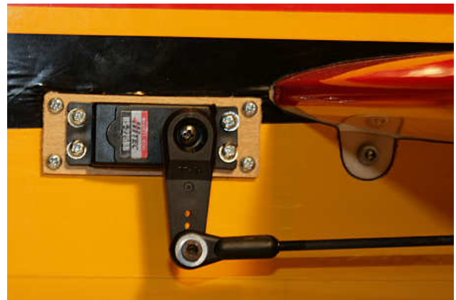
Picture 28: Servo frame / Adaptor
