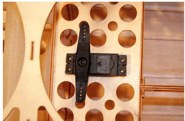
Picture 15: Rudder servo
