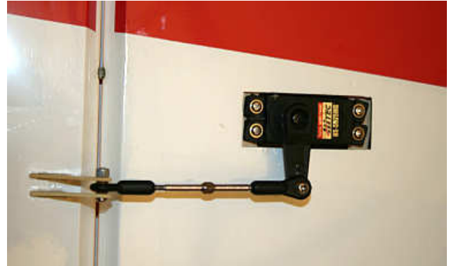
Picture 7: Aileron linking
