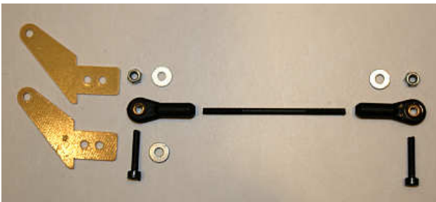
Picture 1: Aileron / Linkage
